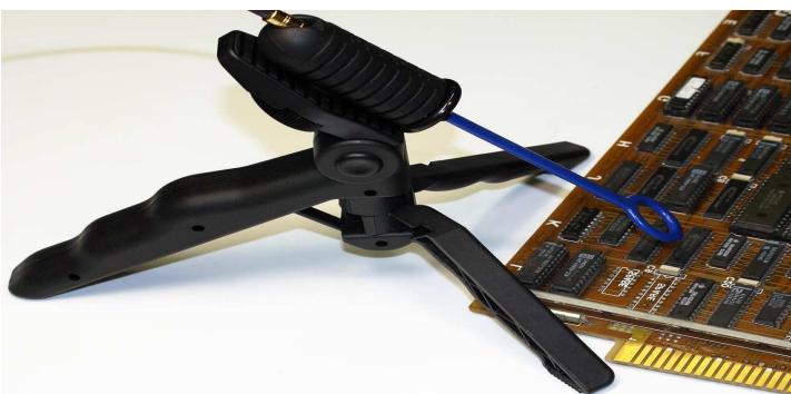
Use of the included tripod for the fixation of the H-field probe
